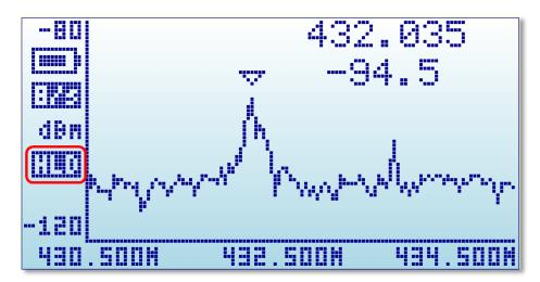
3. The frequency axis now has an enhanced reading with frequency at both ends and also the center frequency. Additionally, you can now cycle between two display modes: LowSpan-Center-HighSpan or Center-Span-RBW. To switch the display mode, click RETURN on the Spectrum Analyzer screen anytime except when it is on HOLD mode.
