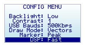
The DSP Auto mode will properly select Filtering or Fast internal modes based on a number of factors as described below. Note the DSP Auto mode is the default every time you start the unit, regardless the mode used in the previous session.
