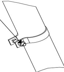
4. Securely attach Clamp, P/N 7749-00, to permanently grounded rod or pipe.
