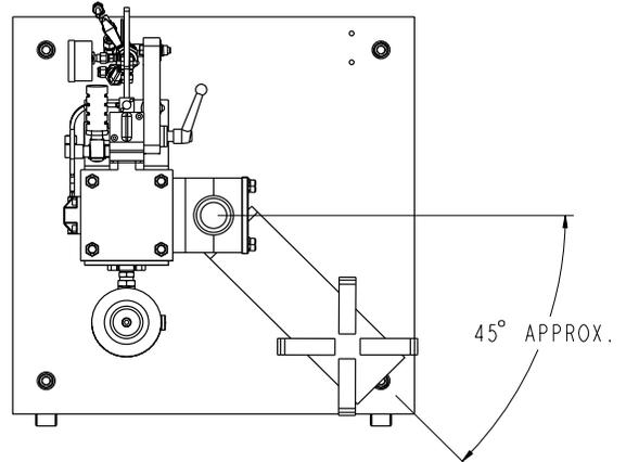
7. Attach air manifold p/n 23555-00 to the air motor.
