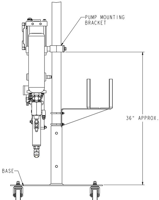
6. Mount catalyst bottle approximately 26" from the top of the base plate, to the bottom of the catalyst bracket.
