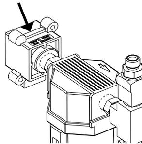
8. Open the air valve p/n 3165 on the solvent tank and adjust the solvent pressure to 90 PSI. (6 BAR) Open the ball valve p/n 18470-05 on the solvent tank. Next open ball valve p/n 23518-00 on the gun to verify that solvent will flow out of the front of the gun thru. the dispense tip, then close the valve.
