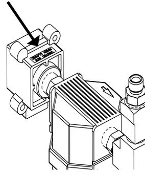
3. Turn catalyst yellow ball valve, P/N 21228-00 to Open / Recirculation position to dump psi. and close the valve.
