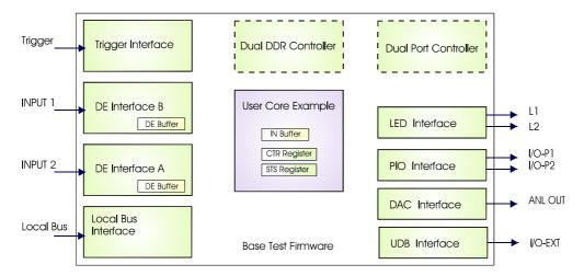
The Base Design is a collection of Acqiris-supplied cores (filled in green on the block diagram) that interface with the underlying hardware of the module.
