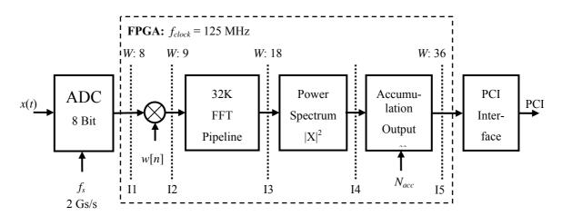
The ADC is shown as a single 8-bit, 2 GS/s converter. In reality, it is implemented with two 1 GS/s ADCs, sampling with a time shift of 500 ps with respect to each other. The 2 ADCs are matched in amplitude, offset, and relative delay through calibration that can be requested with a software command.
