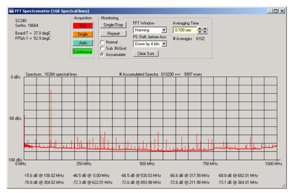
• **Sub BkGnd** displays the power spectrum after the subtraction of a *Background Spectrum*. By default the background spectrum is set to zero.
