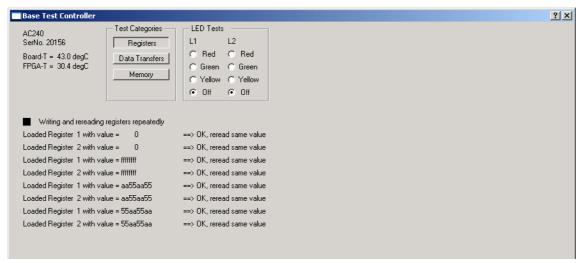
In addition, the control of the front panel LEDs by the FPGA can be tested by pushing the radio buttons in the *LED Tests* section. The LEDs L1 and L2 should show the requested color.
