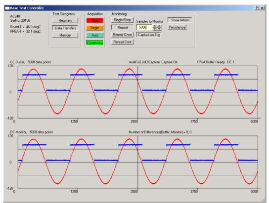
For a detailed analysis of an observed data transfer problem, the **Show Wform** button can be released as shown in the following figure, to display the data in hexadecimal format. When 2 channels are available, the numeric data of Channel 1 are displayed first, followed by those of Channel 2.
