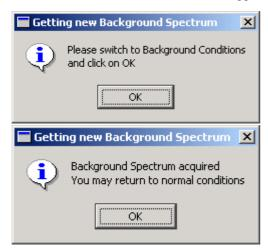
When you press OK after setting your system to a "Background" configuration, the application restarts the FFT operation and acquires a power spectrum in the new conditions. It will be used as the *Background Spectrum*.
