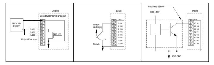
Sinking Output configuration ON or LOW = closed circuit OFF or HIGH = open circuit
