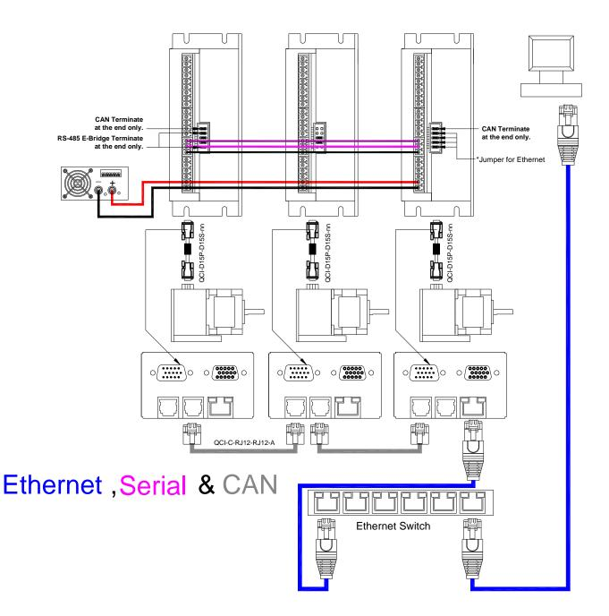
This configuration shows a three-axis system, consisting of one QCI-D2-IG8-E with two QCI-D2-IG8 controllers. The E-485 Bridge provides a bridge between Ethernet and RS-485, providing communications to all 485 connected controllers. One Ethernet connection using one IP address communicates with a whole network of QuickSilver servo controllers.
