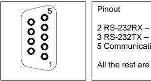
2 RS-232RX - RS-485A 3 RS-232TX – RS-485B 5 Communication Ground
