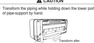
Remove the auxiliary insulation material sheet which is attached to the pipe insulation. Connect the refrigerating pipe.
