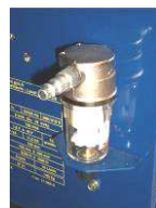
Pneumatic filter, connection to the pneumatic network system
