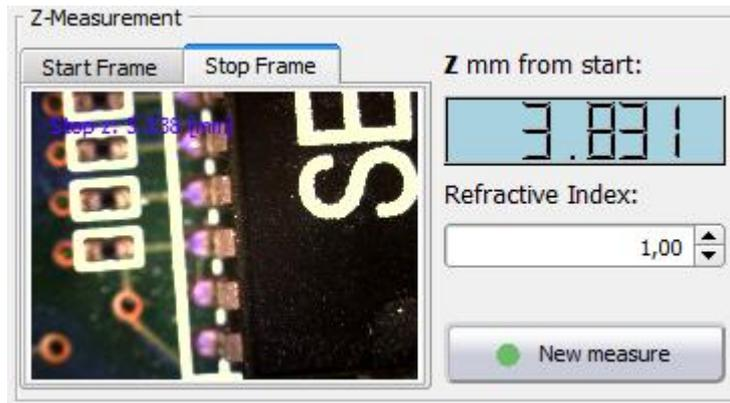
When the stop point is set both the start and stop image can be viewed in the start and stop frame. The distance between the start and stop surface is displayed in the digit field. An image of both the start and stop frame has been saved in the current examination folder. The measurement result is burnt in to the image; an example of such an image can be view below. To make a new measurement, click “New measure”.
