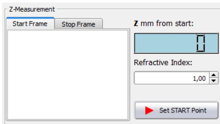
When a start point has been set the start image can be viewed in the start frame and the Z-distance from the start will be displayed in the digit field. The Refractive Index parameter is used when not measuring in air. For example when measuring the thickness of a protection coating you enter the refractive index of the coating in the Refractive Index box. The distance shown in the digit field is always the length read from the measurement instruments multiplied with the refractive index.
