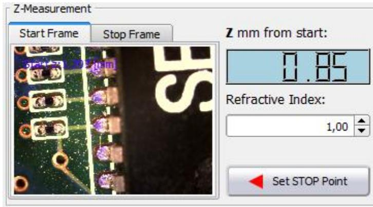
Continue by moving the microscope to set the focus on the surface you want to measure to. While moving the microscope the current distance from the start point will be display in the digit field. When the stop surface is in focus, click “Set STOP Point” to finish the measurement.
