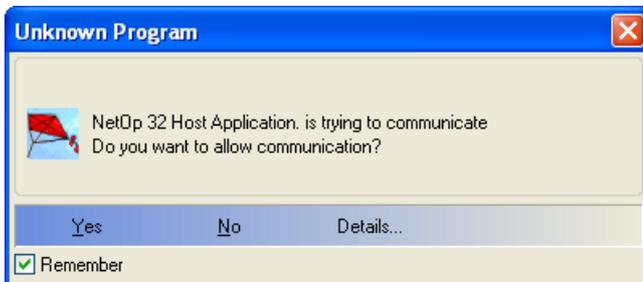
In this example NetOp Host tries to communicate with the network during the initial startup using outbound communication. As such, NPC prompts the user to allow this program to communicate. By checking *Remember* and clicking Yes, this program will be added to the database with the firewall rule Allow Communication.
