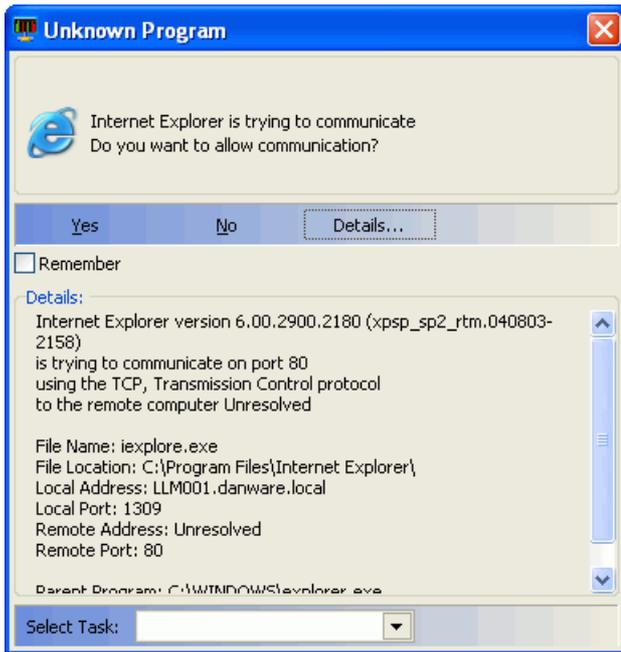
By clicking Yes this program will be added to the database with the firewall rule Allow Communication. The next time Internet Explorer is being launched, the user will not be prompted for a decision.
