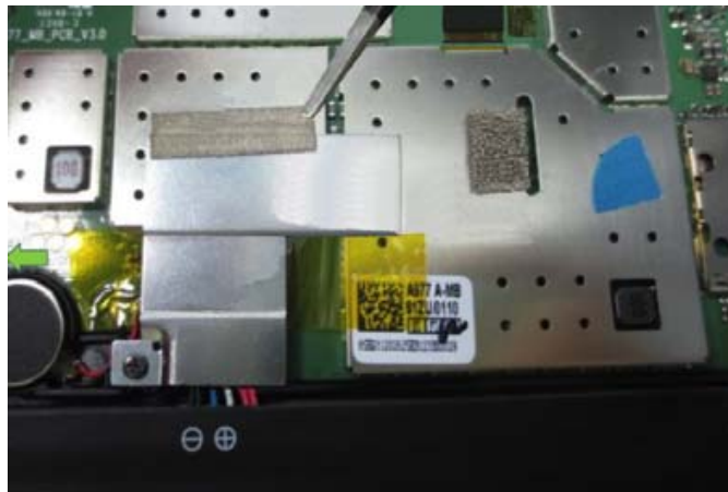
Figure 2-1. The conductive fabric on the steel frame
