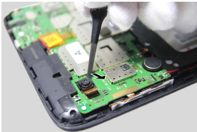
Figure 3-2. Detaching the rear camera
