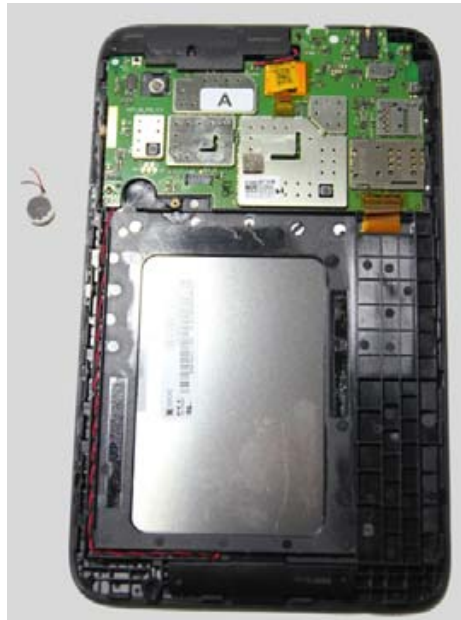
Figure 5-3. The removed vibrator motor
