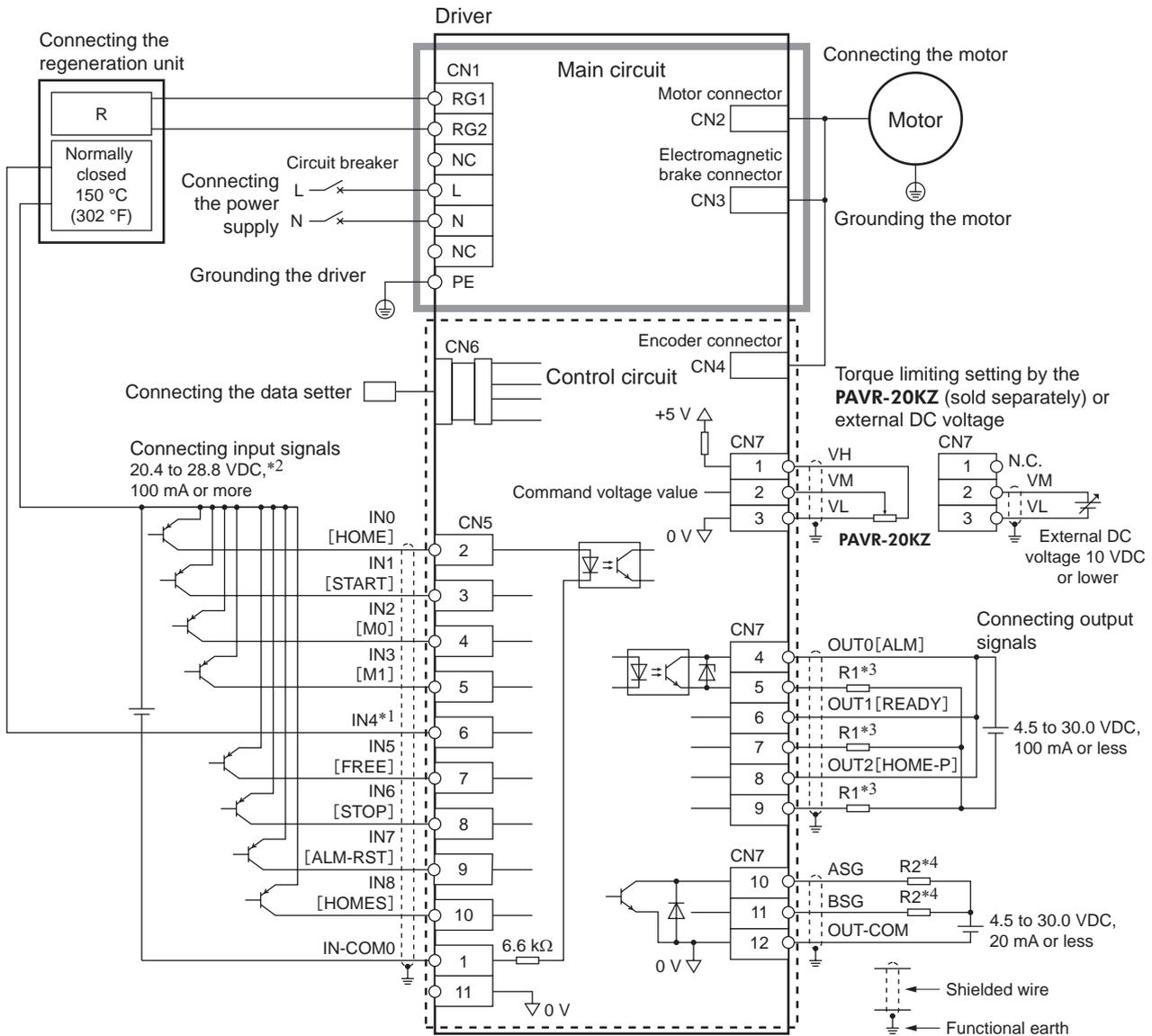
\*1 This is a connection in which the TH input is assigned to the IN4. The initial value is [M2].
