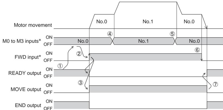
\* Turn the FWD input or RVS input ON after setting the M0 to M3 inputs.
