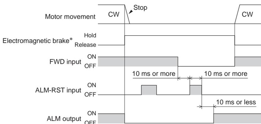
\* The electromagnetic brake will hold the load at the moment an alarm generates.
