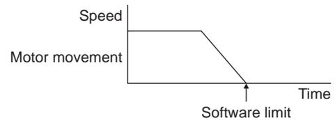
**Note** Software overtravel will become effective when the position origin is being set. See the following for setting the position origin.
