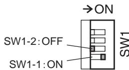
Set the SW1-No.1 and SW1-No.2 to the ON side and OFF side respectively. Position control operation can be performed. Up to 16 operation data can be set.
