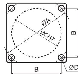
ØC indicates the pilot diameter on the flange.
