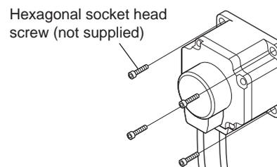
Hexagonal socket head screw set (supplied with the combination type parallel shaft gearhead)
