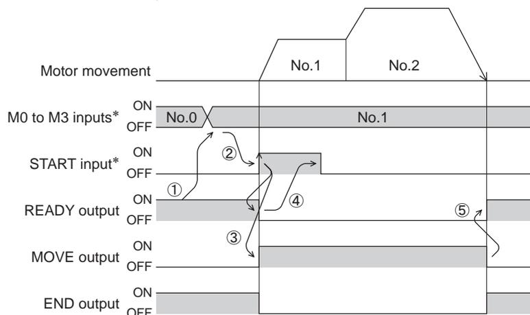
\* Turn the START input ON after setting the M0 to M3 inputs.
