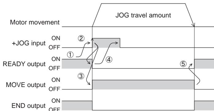
**Note** JOG operation cannot be executed while the FREE input or STOP input is being ON. Be sure to execute after turning OFF.
