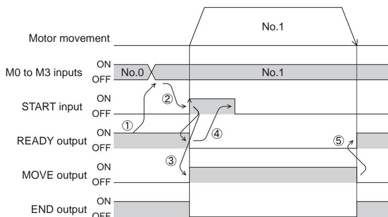
\* Turn the START input ON after setting the M0 to M3 inputs.
