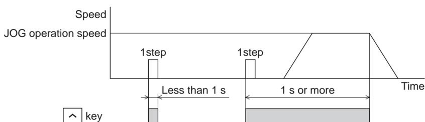
**Note** | JOG operation cannot be executed while the FREE input or STOP input is being ON. Be sure to execute after turning OFF.
