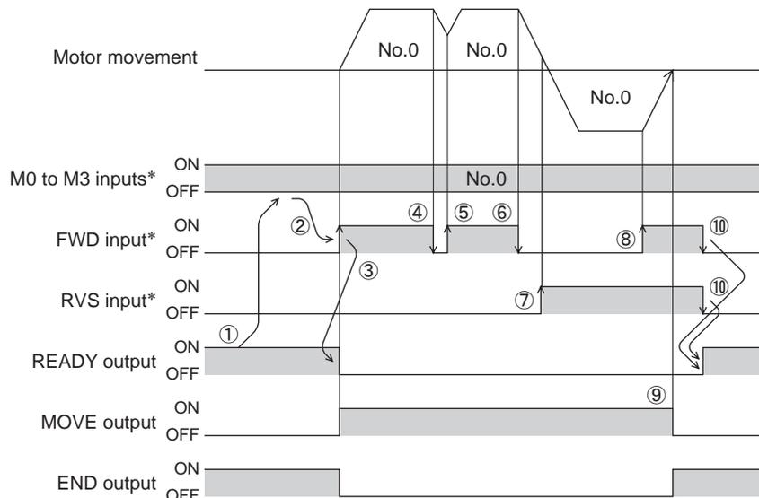
\* Turn the FWD input or RVS input ON after setting the M0 to M3 inputs.
