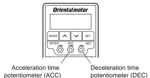
**Note** Be sure not to turn the acceleration time potentiometer and deceleration time potentiometer too much since they rotate lightly. Doing so may damage the driver.
