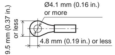
• **Lead wire for Protective Earth Terminal of the motor**
