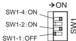
Set the SW1-No.1 to the OFF side, and set the SW1-No.2 and SW1-No.4 to the ON side. When the **BX** Series is used in the speed control mode, the **BX II** Series can be used in similar I/O conditions or functions as the **BX** Series by using this control mode.
