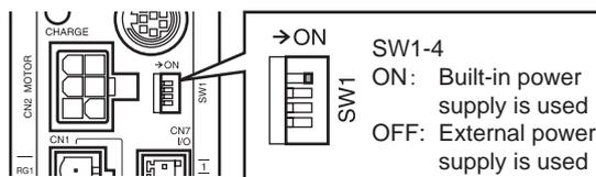
**Note** The built-in power supply cannot be used with the source logic. If the source logic is used, do not set the SW1-No.4 to the ON side.
