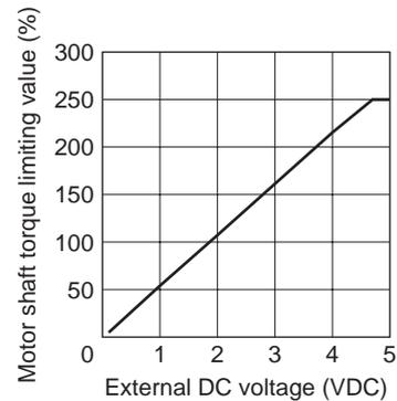
**Note** Be sure to keep the external DC voltage to 10 VDC or lower. When connecting the external DC power supply, make sure the polarities are correct. If the polarities are reversed, the driver may be damaged.
