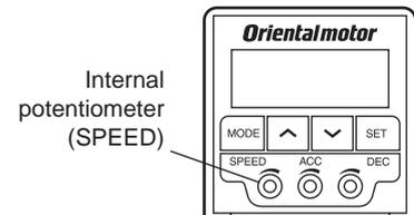
**Note** Be sure not to turn the internal potentiometer too much since it rotates lightly. Doing so may damage the driver.
