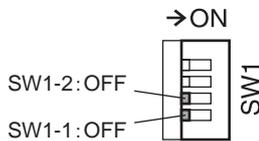
Set the SW1-No.1 and SW1-No.2 to the OFF side. Speed control operation can be performed. Up to 16 operation data can be set.
