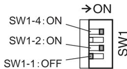
Set the SW1-No.1 to the OFF side, and set the SW1-No.2 and SW1-No.4 to the ON side. When the **BX** Series is used in the speed control mode, the **BX II** Series can be used in similar I/O conditions or functions as the **BX** Series by using this control mode.
