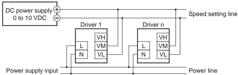
Current capacity (I) of external DC power supply when the number of drivers is n:
