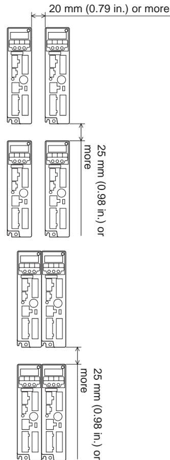
It is possible to install drivers closely in the horizontal direction. In this case, install the drivers to a heat sink [corresponding to an aluminum plate of 350×350×2 mm (13.78×13.78×0.08 in.)].
