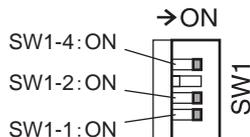
Set the SW1-No.1, SW1-No.2, and SW1-No.4 to the ON side. When the **BX** Series is used in the position control mode, the **BX II** Series can be used in similar I/O conditions or functions as the **BX** Series by using this control mode.
