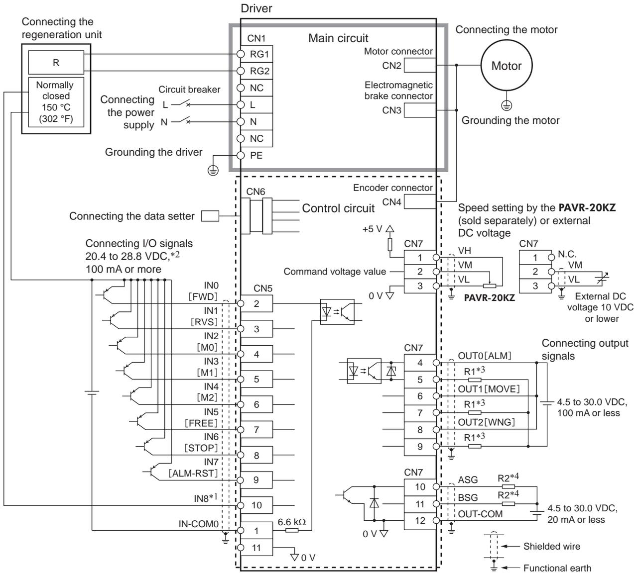
\*1 This is a connection in which the TH input is assigned to the IN8. The initial value is [Not used].
