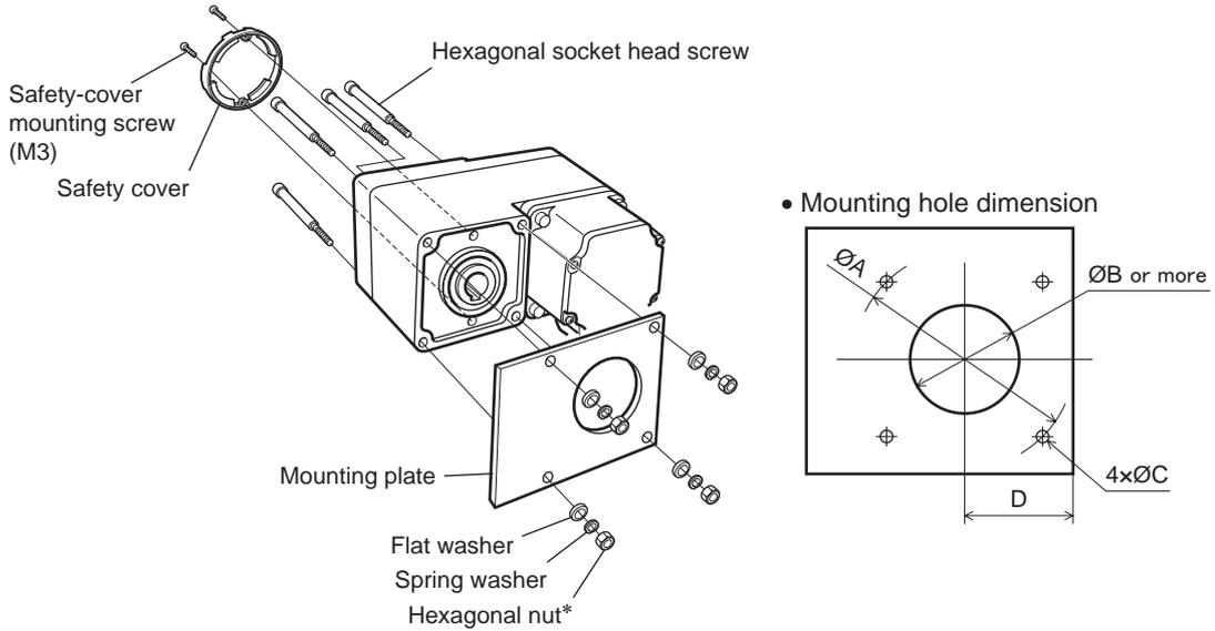
\* The **BXS6200** and **BXS6400** do not come with hexagonal nuts. Provide hexagonal nuts separately or drill tapped holes in the mounting plate.
