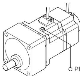
• **Protective Earth Terminal of the motor**
