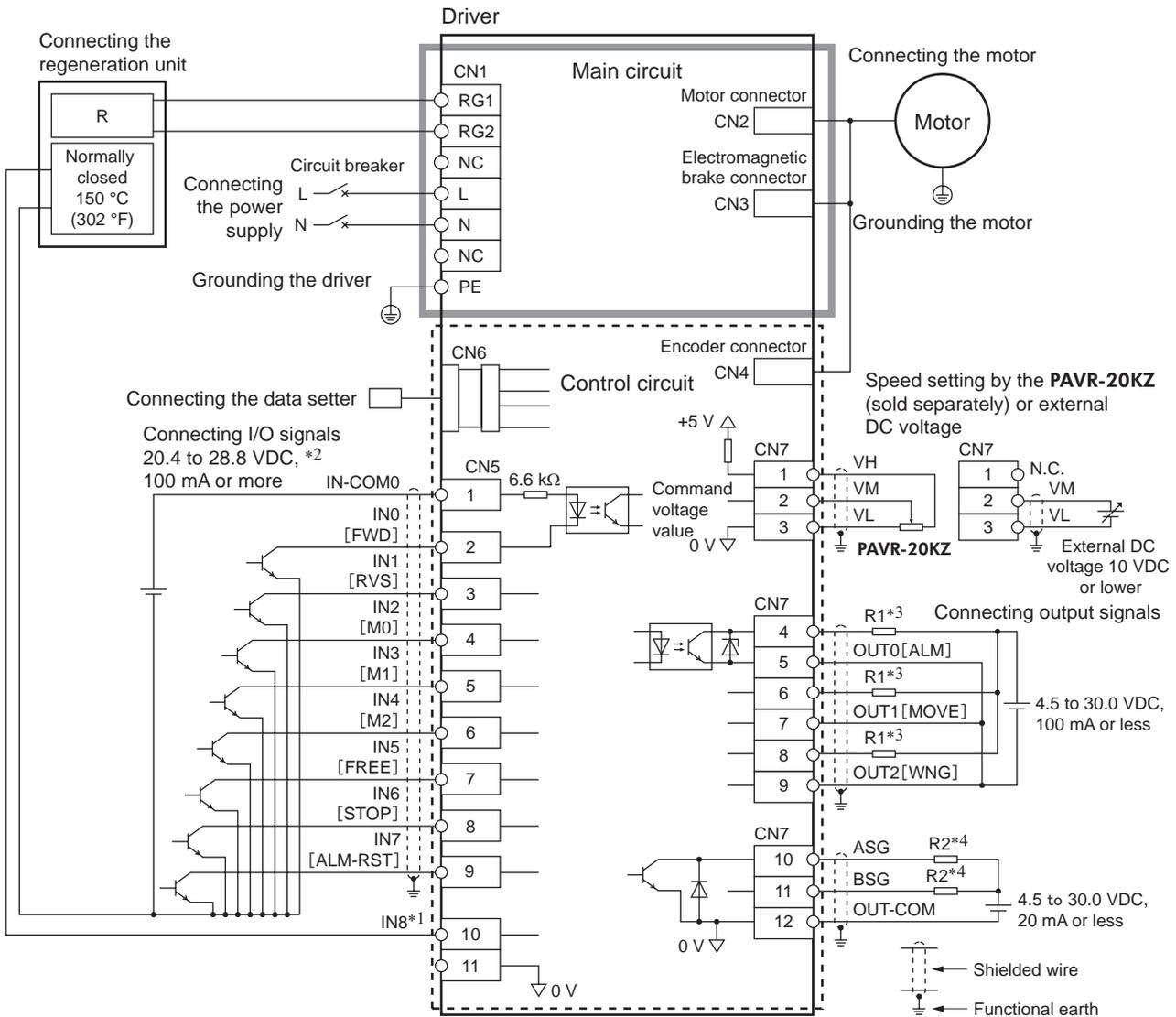
\*1 This is a connection in which the TH input is assigned to the IN8. The initial value is [Not used].
