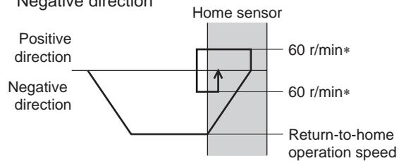
\* When the return-to-home operation speed is set to 60 r/min or lower, the set return-to-home operation speed will be applied.
