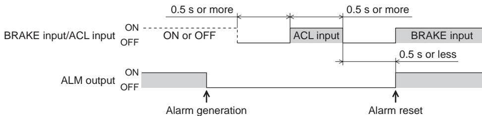
**Note** Some alarms cannot be reset with the ACL input. To reset these alarms, cycle the power. Refer to p.154 for details.
