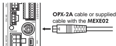
**Caution** The data edit connector (CN6) and I/O signals connector (CN5/CN7) are not electrically insulated. When grounding the positive terminal of the power supply, do not connect any equipment (PC, etc.) whose negative terminal is grounded. Doing so may cause the driver and this equipment to short, damaging both.
