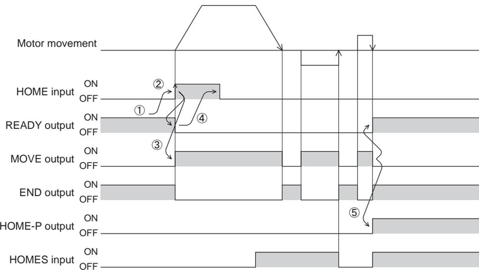
**Note** Return-to-home operation cannot be executed while the FREE input or STOP input is being ON. Be sure to execute after turning OFF.
