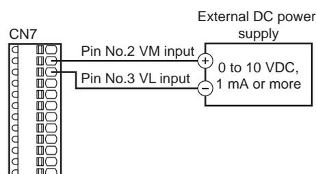
**Note** Be sure to keep the external DC voltage to 10 VDC or lower. When connecting the external DC power supply, make sure the polarities are correct. If the polarities are reversed, the driver may be damaged.
