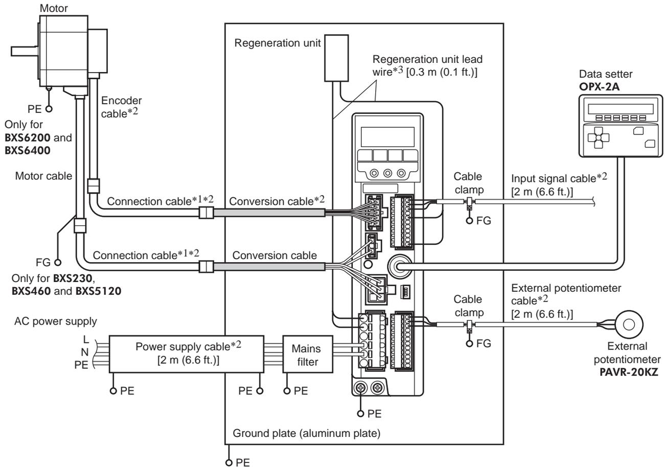
\*1 Up to 30 m (98.4 ft.) of the connection cables have been evaluated. The connection cable can be connected up to 2 pieces.
