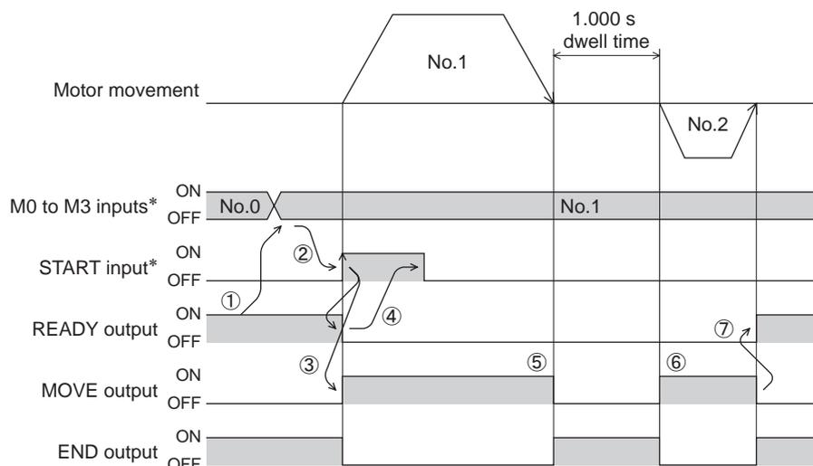
\* Turn the START input ON after setting the M0 to M3 inputs.
