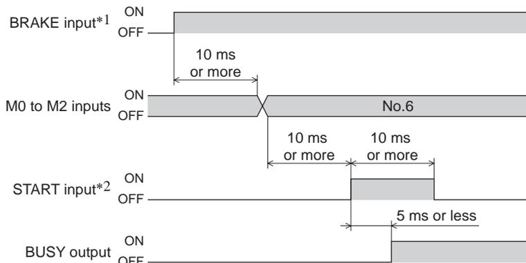
\*1 Be sure to turn the BRAKE input ON before operating the motor.
