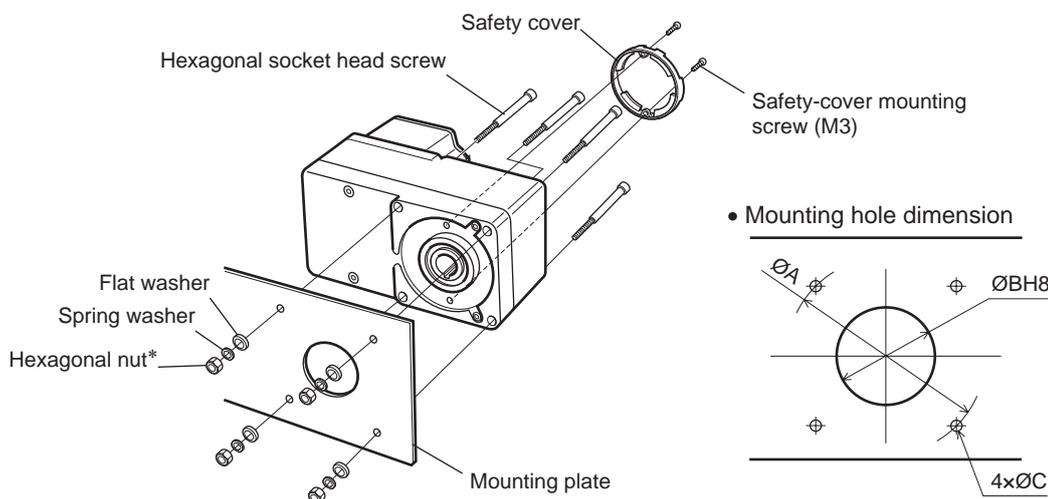
\* The **BXS6200** and **BXS6400** do not come with hexagonal nuts. Provide hexagonal nuts separately or drill tapped holes in the mounting plate.
