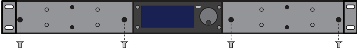
Figure 2.4 Screw Locations on Each Power Supply
