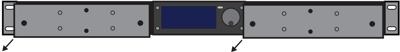
Figure 2.5 Removing the Power Supplies from the Chassis
