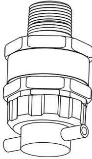
Figure 11. MPD with Flow Adaptor
