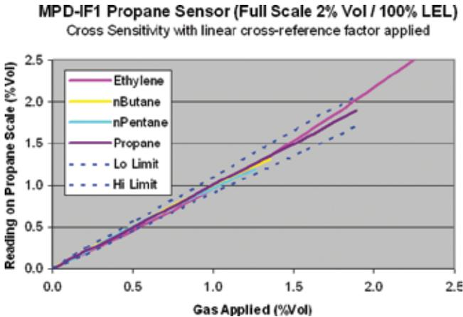
Figure 12. MPD-IF1 (Propane) Sensor with linear cross-reference factor applied
