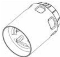
Figure 4. Weatherproof Housing
