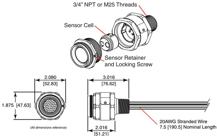
Figure 1. Multi-Purpose Detector (MPD)
