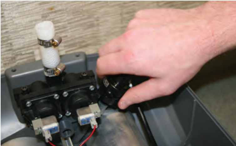
Figure 17: Showing Connections to Pressure Regulator
