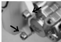
6. If you use a thru-axle hub you **must** use thicker 3mm spacers. These are either available separately (code: 0720 829) or come supplied with the MAGURA Gustav M thru-axle hub. If necessary you might have to use here as well additional 0,2mm spacers for a clean and drag free positioning of the caliper.
