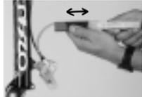
7. Press the MAGURA BLOOD oil through the system. Use a second syringe to suck any overflowing oil at the reservoir. Then pull the filler syringe to suck oil back. Repeat procedure 3-4 times and actuate **CAREFULLY** the lever blade simultaneously. **Make sure that there is always enough oil in the reservoir when you suck the oil with the filling syringe!**
