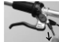
8. Always check for correct installation by pulling on the hose. Make sure that the system has no leaks. Squeeze the lever blade, hold pressure and check hose connections and the reservoir cover for eventual leaks. Squeeze the lever blade several times (pump) to push the pads to their proper position until the lever feel becomes very firm. If you cannot realize this, bleed the brake (see page 15 onwards).
