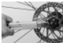
8. Mount the rotor with the 6 Torx T25 bolts onto the hub. Watch out for the correct rotation direction of the rotor (laser arrow). Use only new original bolts or thread lock if you use old bolts. **Tighten the bolts in a crossed pattern! Tightening torque: 4Nm/34 in.lbs.**
