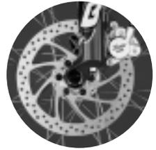
Brake caliper and rotor
