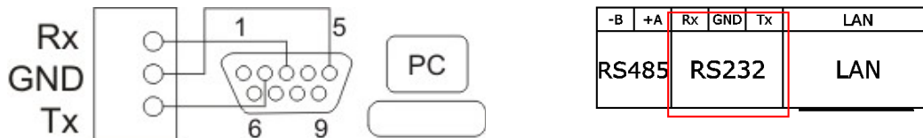
Picture 13. Connecting over RS232
