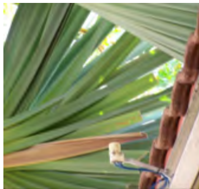
Figure 56. Rain sensors installed in places where normal rainfall is likely to be obstructed.
