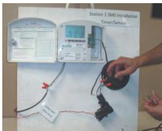
Figure 58. A demonstration of proper wiring of a soil moisture sensor.
