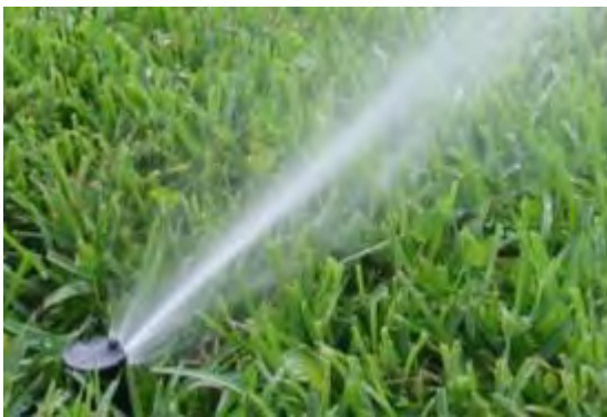
Figure 45. Rotor used to irrigate open areas of turf.
