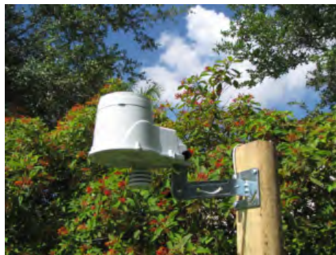
Figure 60. An advanced climate sensor for a smart irrigation system.
