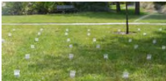
Figure 62. A catch-can test used to determine distribution uniformity.
