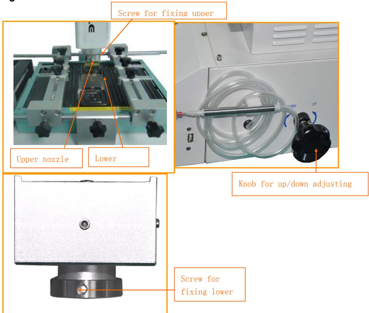
2. 3.Adjust upper and lower nozzle positions; rotate the knob to lower the upper heater; by moving upper heater backward/forward, make the centre of upper nozzle and lower nozzle align. After adjusting, lock the forward/backward handle and fix the heater not moving forward/backward. Then lift the upper heater. If need to rotate upper heater, loosen the upper heater rotate lock. If not, tighten it.
