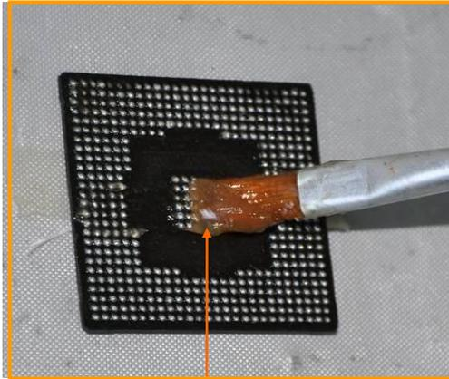
Apply solder flux with brush
