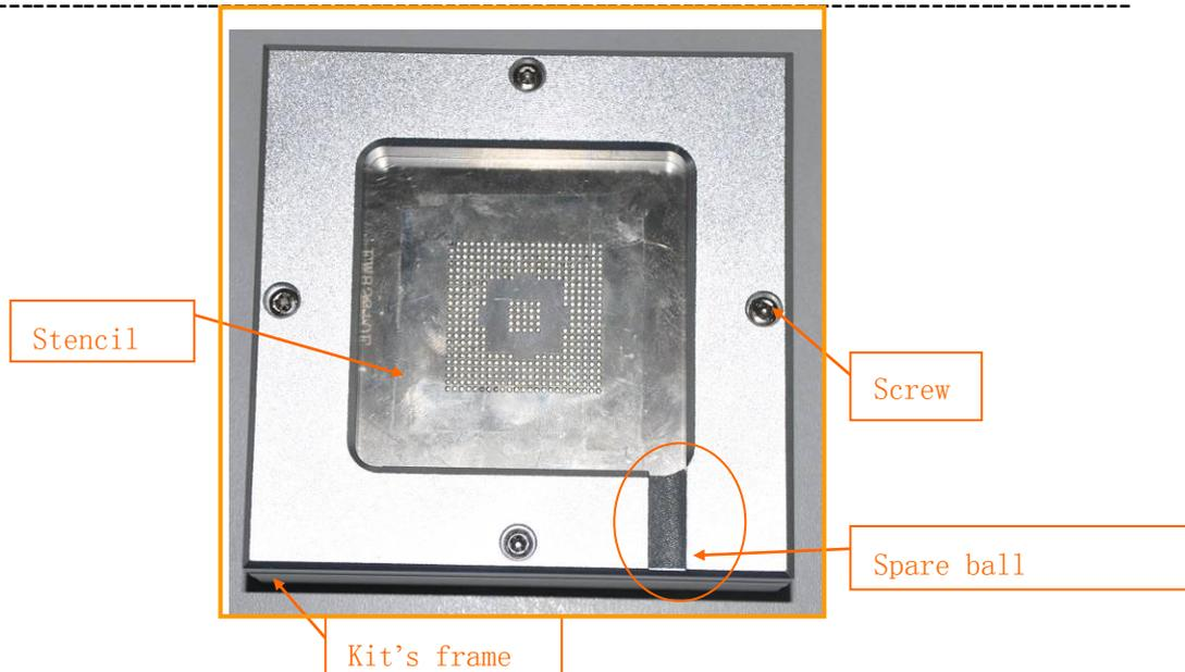
5.2 Apply solder flux to BGA equally, then place BGA as the picture showing below; adjust the locating block to make BGA's diagonal and the reball kit's diagonal match together, only in this case the BGA is located in the center of the reball kit; finally lock the four locating block it fix it.
