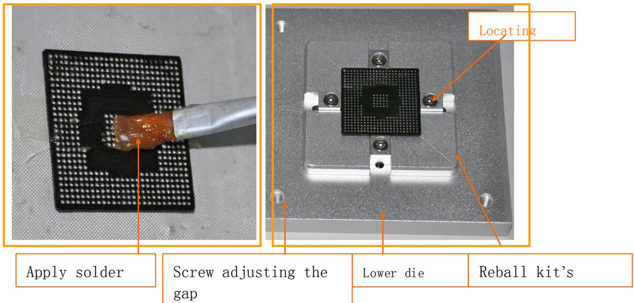
5.3 Put the cover with stencil inside over the kit; then move the stencil lightly to make its holes match the BGA pins. In case this method is not good enough to make stencil's holes and BGA pins match each other, (pay attention to the deviation place) remove the cover(frame), release the screw, readjust BGA and repeat all
