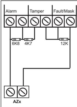
ELF1 wiring is used for detectors that have a relay output (a pair of terminals) for Fault or Mask.
