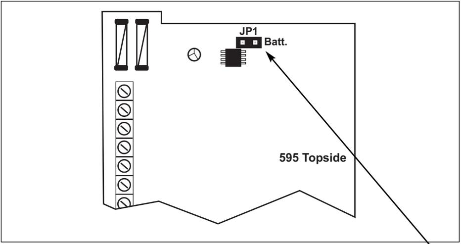
If powering up the Control Panel with battery only, connect battery and short out **JP1** for approx. 5 seconds. Key pad and Control Panel will then become active.
