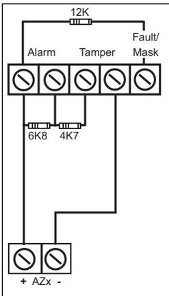
ELF2 wiring is used for detectors that have a transistor output (a single terminal) for Fault or Mask.
