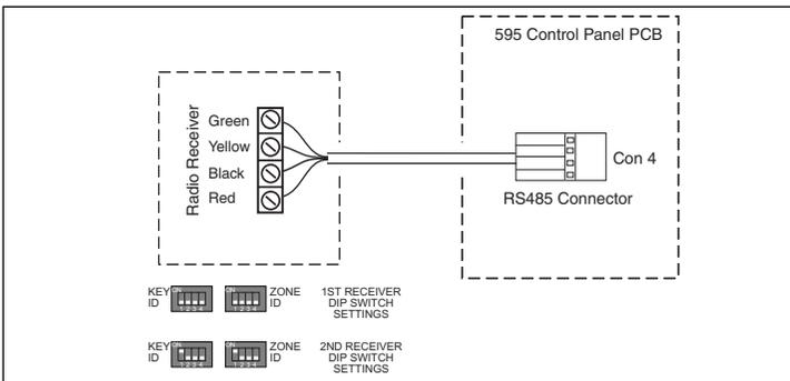
Connect cable between **Con 4** on the 595 PCB and the Radio Receiver.
