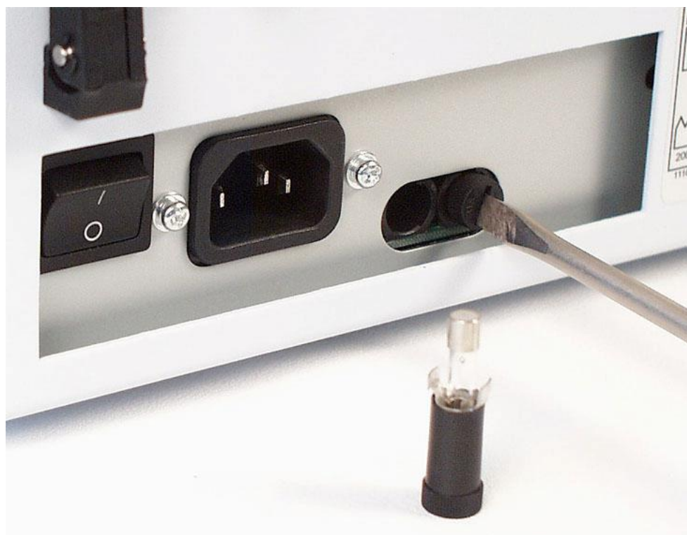
Fig. 7.8 Changing the fuses
