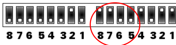
Fig. 5.13 DIL switch positions 5, 6, 7 and 8 for transmit / receive selection
