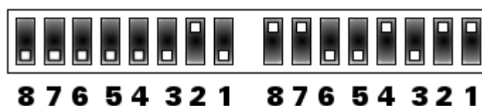
Fig. 5.10 Factory set DIL switch positions, viewed from the rear as shown in Fig. 5.9.
