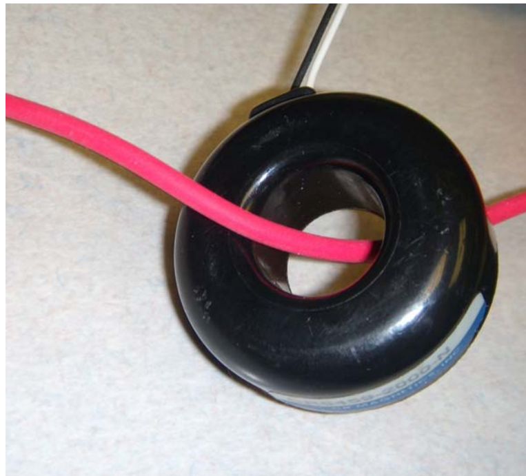
Figure 2. AC Load Wire Installed in CS10 (colour of ac load wire can vary)
