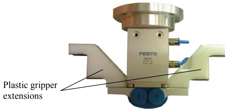
Fig. 2b. Pneumatic gripper in its opened position.
