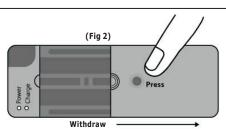
Once the Slippery board is blocked at 50mm, you could extend it with adding 5mm by pressing the circular button and withdrawing. By this action, the maximum extension becomes 55mm and fit with more battery's sizes (as shown in Fig2)
