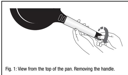
Hold the handle with one hand and twist the black end tip of the handle with the other hand counterclockwise. If necessary, use a thin, long, sturdy object such as the handle of a wooden spoon or skewer and push it through the hole in the tip of the handle to act as a lever to assist you with twisting.
