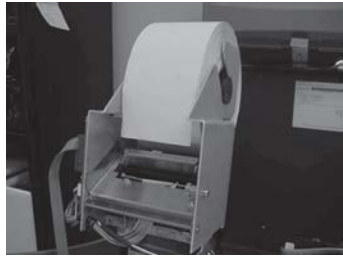
Figure 6-6. Paper feeds from top of roll.
