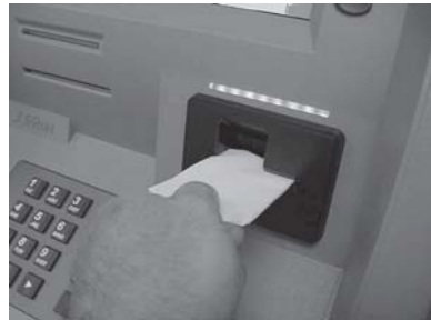
Figure 6-11. Use the cleaning cards on a monthly basis to maintain effective card reader operation.
