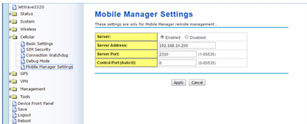
Between the Mobile Manager Server and Remote Cellular Devices, it is complex and different environment may have different requests. The Public IP and open specific TCP port for your Mobile Manager Server are MUST settings. You can check the public IP address with your carrier provider. Normally, you must pay the cost to keep the permanent public IP. After you have the public IP, you must open the
