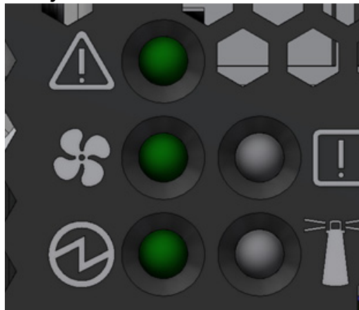
Figure 21: System Status LEDs 5 Minutes After Power On
