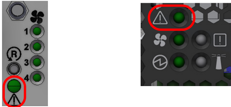
Figure 25: System Status LEDs - Front and Rear sides
