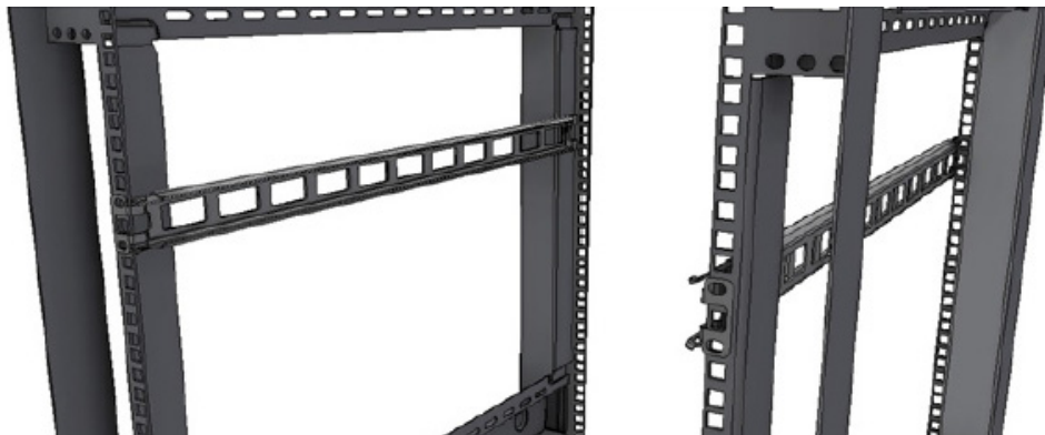
Figure 14: Mounting the Outer Rails into the Rack
