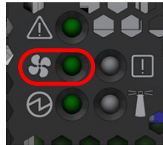
Figure 26: Fan Status LED - Front and Rear Sides
