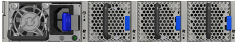
Figure 24: Fan Module Latches
