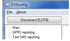
When the module *G10* is connected to a computer, module LED *Power* should flash green and yellow in turn. Program *G10config* status bar should indicate connection status as *Connected* and the following information about the connected module:
