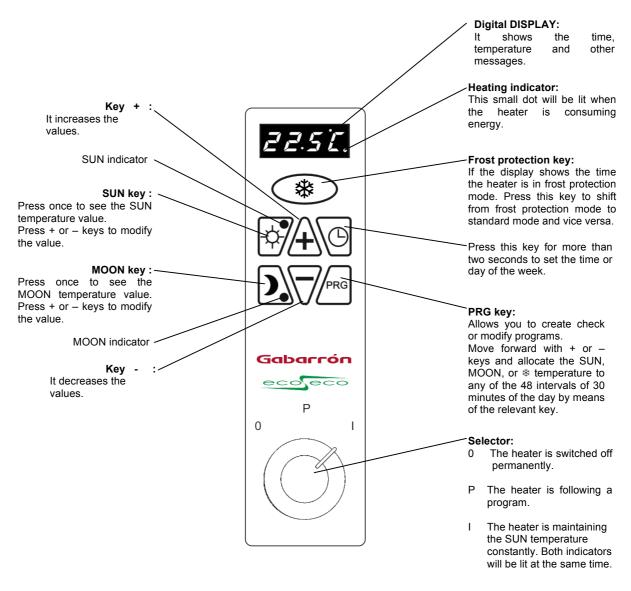
Digital models have built in an electronic thermostat with a sensibility of 0.1 °C. It is possible to set temperatures with an accuracy of 0.5 °C.
