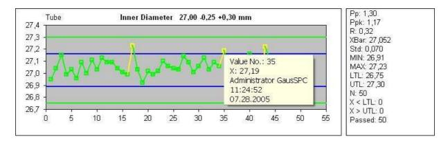
The X or pre-control chart displays single measurements in the order they were recorded. For each measurement there is one point on the graph.
