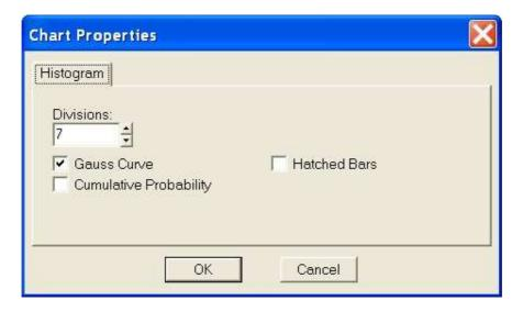
You can set the number of divisions, display of the Gauss curve and the Cumulative curve. The bars can either be coloured or hatched. For details of how to set colours, please see Section 7.5.
