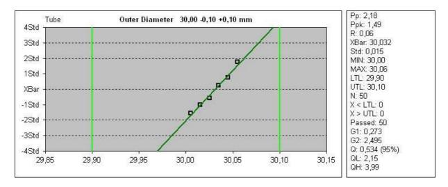
The probability plot is different from the histogram in that instead of number of meawsurements in a single division on the vertical axis, there is a cumulative frequency by divisions expressed in terms of standard deviation. From this chart it is possible to quickly see the average value and ratio between the range and the tolerance field.
