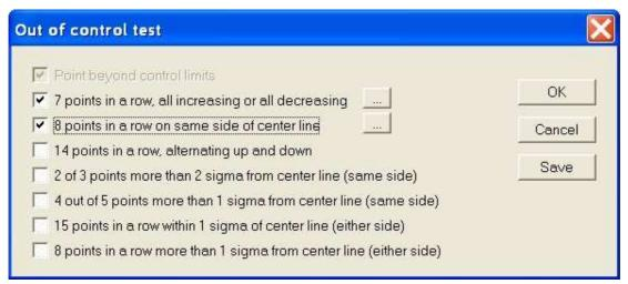
Click on the Browse button next to the 'x points in a row, all increasing or decreasing' and the 'x points in a row on same side of centre line' in order to amend the number of points which should be taken into account.
