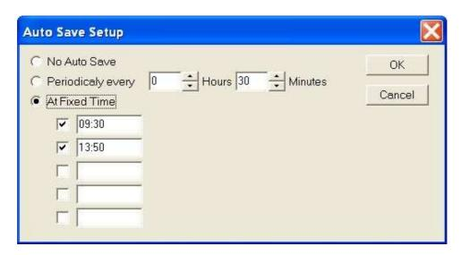
GausSPC can either save measurements periodically after a defined interval or at certain times e.g. at the end of a shift. The shortest save interval is ten minutes.
