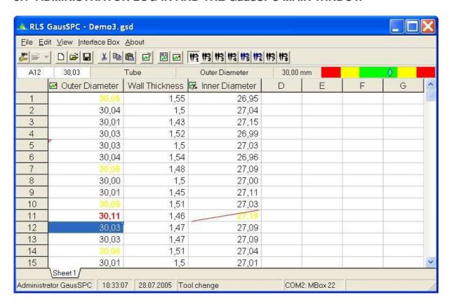
Above is a typical GausSPC main window with a worksheet containing measurements, the menu, toolbar and two status bars. The cursor (the blue coloured active cell) is moved through the sheet using the arrow keys, PgUp, PgDn, Home and End keys. The screen view can also be moved by using the scroll bar on the right of the screen.
