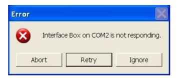
If the error message repeats even though you have checked the above criteria, click the Ignore button, continue with log-in and then in the main window repeat the selection by selecting Interface Box/Setup.
