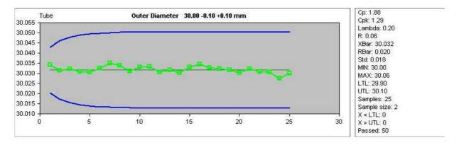
In addition to the statistical parameters already described for X-chart and histogram, the Lambda parameter, sample size and number of samples are also added to the list of statistical parameters.
