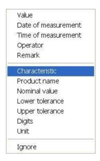
If a single line contains measurements for more than one characteristic (with 'All Characteristic Data in one line' unchecked) you will have a shorter list of available information types.
