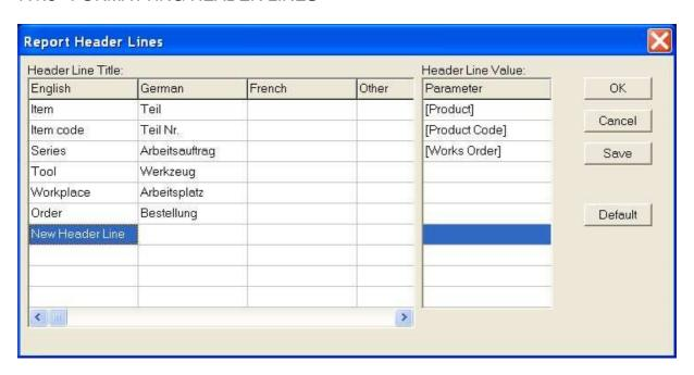
To display the Header Lines dialog box, double-click in the Header Lines area on the report or select Text / Header Lines from the menu.
