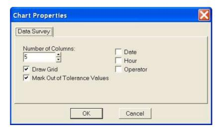
For X-R, X-s and EWMA charts measurements are grouped by samples. Two columns are also added which display the average value and range.
