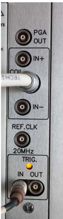
4. The “PGA OUT” output (“PGA” = “Programmable Gain Amplifier”) can be used to monitor the coil signal, after input filtering and amplification, just before analog-to-digital conversion.
