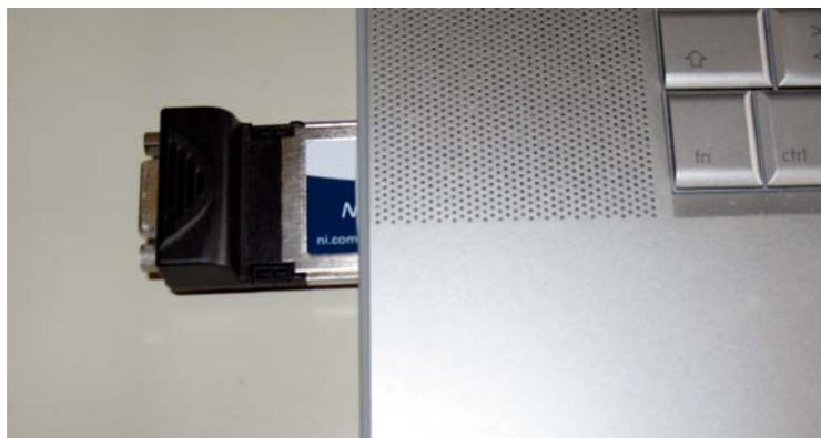
2. Connect the cable between the bridge cards in the computer and the crate.
