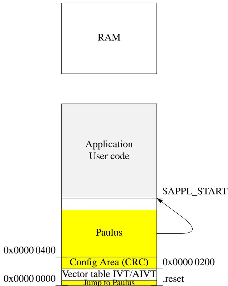
The APPL\_START value is set with 0x4000 which allows an easy implementation with debugging and a great number of printf output. After doing own adjustments it is possible to optimize this value to get more space for the application.
