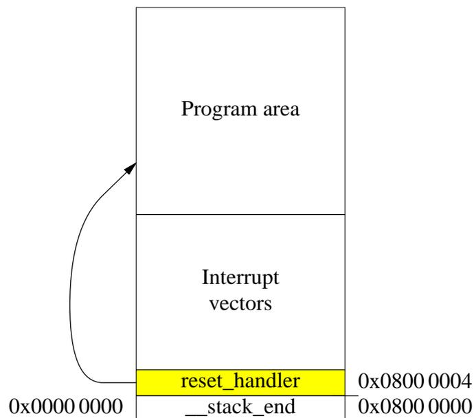
In order to start the application correctly it is necessary to set the *define* `STARTUP_FROM_RESET` when compiling `STM32_Startup.s`. Otherwise, at least CrossWorks compiles a loop as the *reset\_handler* called `reset_wait` to give a Debugger the chance to stop execution at a defined location.
