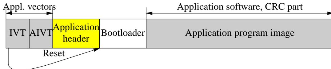
The bootloader checks the received data by a CRC checksum. Therefore an application header of 128 byte is necessary. This header can be generated with the tool **paulus\_cksum** and contains the following information as described in chapter 7 APPLICATION\_HEADER\_T.
