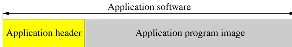
The Bootloader checks the received data by a CRC checksum. Therefore an application header is necessary. This header can be generated with the tool **paulus\_cksum** and contains the following information as described in chapter 7 APPLICATION\_HEADER\_T.
