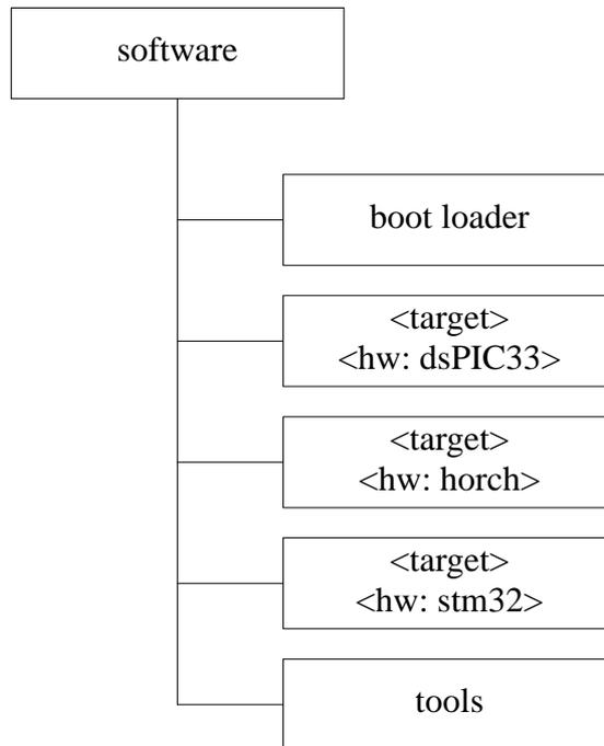
The directory *bootloader* contains the hardware independent part of the software. The hardware dependent part of the software is named after its hardware, e.g. *horch*. Configuration is stored in the *horch*-directory. Projects and *main.c* are stored in *software*
