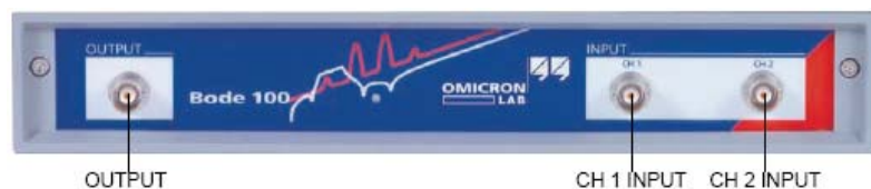
Fig. 2: Bode 100 front view
