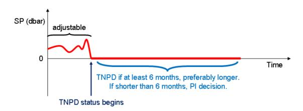
Example (d). The time series starts with a continuous zero-reading period, then reverts back to valid positive values. The initial zero-reading period does not qualify as TNPD. This is because pressure drifts are typically monotonic and therefore a reversal back to positive values indicates that the pressure sensor is not likely to have developed a negative drift.
