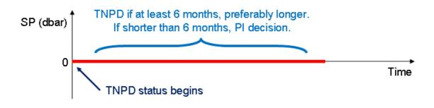
Example (b). There are occasional valid positive SP readings in the first part of the time series, followed by a continuous zero-reading period that does not contain any occasional valid positive readings.
