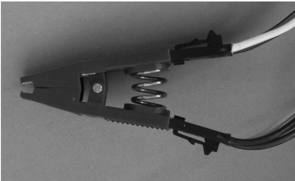
Correct installation of extension cables to Pomona clip
