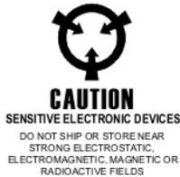
MOS devices are designed to operate at very high impedance levels for low power consumption. As a result, any normal static charge that builds up on your person or clothing may be sufficient to destroy these devices if they are not handled properly. When handling such devices, use precaution to avoid damaging them as described below:
