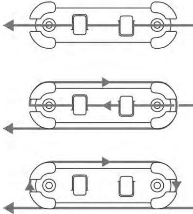
Use the cable clips to secure and manage the cables. You can wrap the excess cable around the security clip to reduce the cable length.
