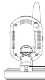
Connect the power adapter to the DC5V port
