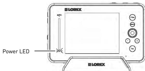
The power indicator LED glows green when the monitor is powered on. When the battery is low, the power LED blinks.
