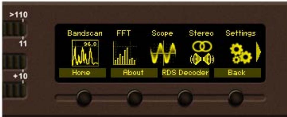
The device settings are organized as hierarchical tree menu (*Settings menu*). Similar parameters are grouped in sections (branches). The overall view of the *Settings menu* is shown on the figure below.
