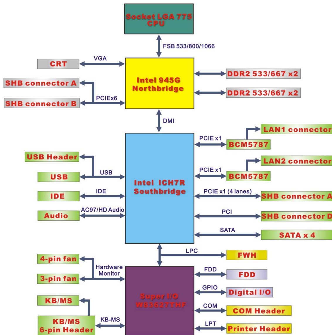
Figure 2-3: Data Flow Block Diagram
