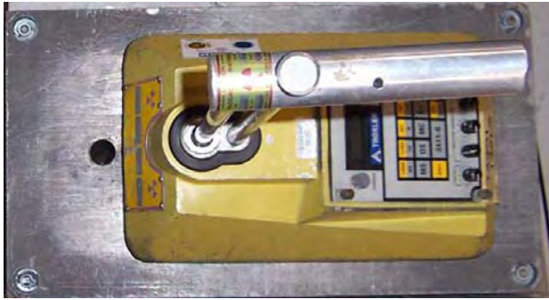
Top view of a Model 3411-B on the magnesium calibration block in backscatter position
