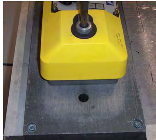
Left side view of a Model 3430 on the magnesium block in backscatter position
