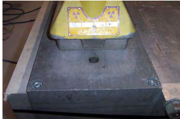
Back view of a Model 3411-B on the magnesium block in backscatter position
