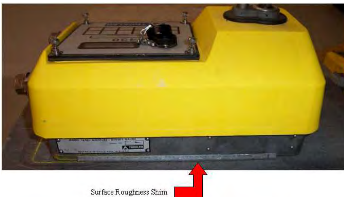
Figure 2–4. Location of Surface Roughness Shims (Note: There is one shim on each side of the gauge.)
