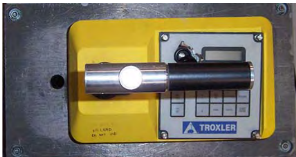
Top view of a Model 3430 on the magnesium calibration block in backscatter position
