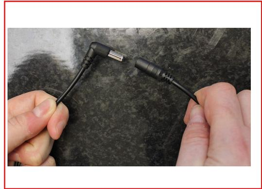
4. Take the permanent power lead and plug it into the DC plug on the power supply provided. Please DO NOT plug the power supply into your power source at this point.
