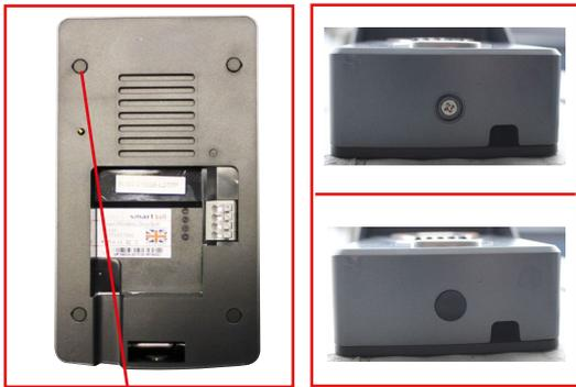
7. Put the screw cap covers in place over the screws at the back of the smartbell. Attach the smartbell to the bracket. Secure the unit to the bracket using the provided screw and place at the bottom of the unit. Then use the cap to cover (shown above, right).
