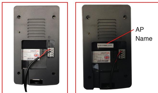
4. Push the red/black cables of the permanent power lead through the hole in the wall and connect to the back of the smartbell. The red wire into the number 1 slot and black into the number 2 slot. To do this, push and hold the grey clip in while pushing in the red/black cables. When pushed in, release the clip to secure the wire.
