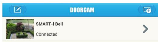
10. Press on the picture to view the smartbell camera and also listen through the microphone to check that you are connected.
