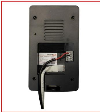
7. If you choose a wired connection to your router/home plug/switch, run your ethernet cable through the hole and connect to the back of the smartbell. Attach as shown above. If you choose a wireless connection skip this step and proceed to step 6.
