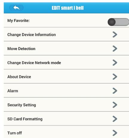
2. Press the 'Change Device Network Mode' option and press the SSID option. The smartbell will search for wireless routers.
