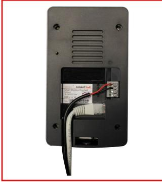
5. If you choose a wired connection to your router/home plug/switch, run your ethernet cable through the hole and connect to the back of the smartbell. Attach as shown above. If you choose a wireless connection skip this step and proceed to step 6.
