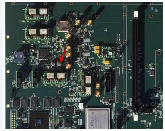
This button has nothing to do with the power monitors or power on. All it does is assert the USER\_RESETn signal to the FPGA (FPGA\_USER\_RESETn\_A, active-low, connected to user FPGA pin AH35). It can (and should) be used as a general-purpose logic reset in the user FPGA design.
