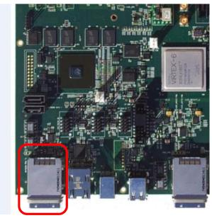
The device appears as three 1MB memory regions to the host machine. You are expected to use the Emu software and drivers (source code provided) to interface with PCI Express. There is no description available of the function of DNV7F1A as a PCI Express device.
