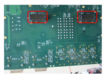
A detailed electrical and mechanical spec, including the connector pin-out, signaling levels, routing rules, mechanical requirements, and connector part numbers, is provided for the DNSEAM\_NS interface, please find it on your board support package. If you are designing a custom DNSEAM\_NS card, it must comply with the DNSEAM\_NS spec. We provide design reviews for DNSEAM\_NS expansion boards, inquire please send requests to support@dinigroup.com
