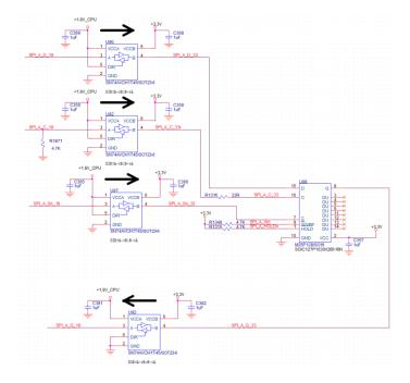
The chip used is Micron M25P128, with 128Mbits of storage space. The interface is SPI. The SPI signals on the FPGA are +1.8V, and are translated up to +3.3V. When calculating timing for this interface please be sure to account for the delay added by the TI SN74AVCH1T45 level translators.
