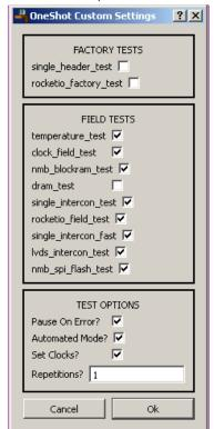
The tests that you can run now are the temperature test, clock test, blockram test, intercon test, lvds test and flash test. Let's skip the DRAM test and the "factory tests" for now. After you hit the
