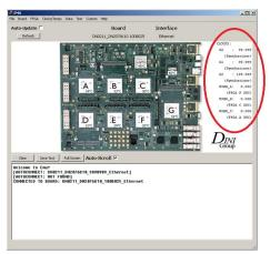
The clocks GO, G1 and G2 can also be set to distribute a signal from an external source. Note that the Si5326 cannot accept input frequencies lower than 2kHz. For very low input frequencies you may consider using the user FPGA SMA inputs described in section 3.3.4.
