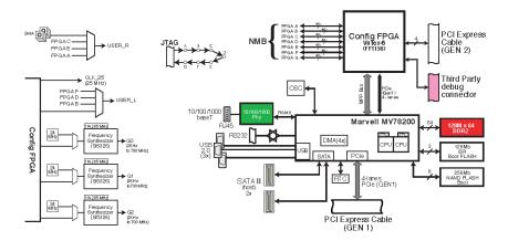
The primary purpose of the Marvell processor is to pump data from a host interface (PCI Express, Gigabit Ethernet, SATA, Flash, or USB) to and from the user's design in the FPGA.
