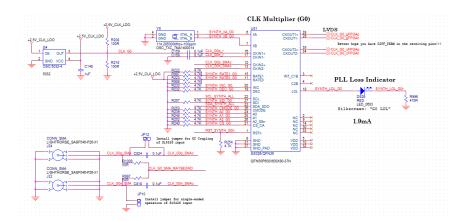
The synthesizer used is a high-performance, low jitter, high-precision clock generator chip, the Si5326. To change the clock frequency you can use the EMU software.
