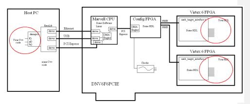
If you want to implement your own software that uses EmuLib to talk to the board from the host PC side, you are expected to understand and use the interface provided by the file diniboard.h (See the software Emu User Manual for details), found in the user package. On the FPGA side, you are expected to understand and use the interface provided by the file nmb\_user\_interface.v also found in the user package. See documentation here:
