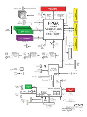
The board contains one Xilinx Virtex-7 FPGAs in the "FF1761" package. There are 5 different Xilinx part numbers that come in this package, the VX330T, VX485T, V585T, VX690T, and V2000T. All 5 of these are compatible with this board (in any speed grade) although the 10Gbps interfaces can only be used with -2 speed grades and faster.
