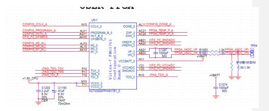
You can also read back the voltages on these pins, the FPGA temperature, and the VCCINT and VCCAUX voltages using IMPACT and the JTAG chain, or by instantiating the XADC block in your design. See Xilinx <u>7 Series FPGAs XADC User Guide</u> (UG480) for details on using XADC functionality within your design.
