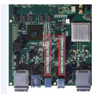
The single "host" interface is intended to be used as a connection to a host PC that will be used with the provided "EMU" software. You are expected to use the EMU controller library to interact with this device.
