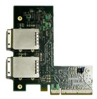
The board fits into any 8x or 16x PCI Express slot. Make sure the computer is powered off when you install the board into it. There are two x4 cable connectors on the board. You should use only the bottom one with the DNV7F1A because the DNV7F1A PCI Express interfaces only support 1x or 4x PCI Express links. The top connector on the PCI Express cable adapter card is for use with 8x links.
