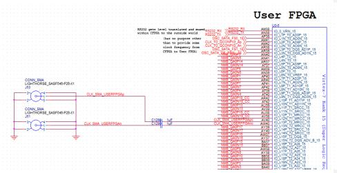
There is no defined purpose for this input. Given that it is on an MRCC pair it is possible that it would be useful for sending a clock into the user FPGA.
