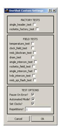
All of the check boxes are tests on the board that can be run independently. The items in the "Factory Tests" area all require specialized test fixture hardware to pass, so they will be of limited use to users for testing the board. The tests in the "field tests" area can all pass without special test fixtures. Note that the DRAM Test requires that there is a DDR3 DIMM (any density) installed in the DIMM slot on the board. If it is not installed, the test will fail.
