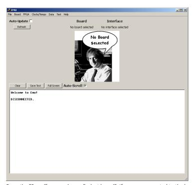
From the "Board" menu, choose "select board". If you are connected to the board over PCI Express, USB and Ethernet simultaneously, then there will be three options in the pull-down menu. Each interface is treated like a separate board. From the pull-down menu, you can see the serial number of each board. The serial number in this menu should match the serial number located on a sticker near DIMM D of your board.
