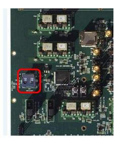
The above photo shows where one might install a battery on the DNV7F1A. The DNV7F1A comes with a battery installed that will last for quite some time.
