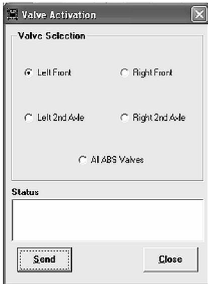
The Valve Activation test screen lets you activate the HPB valves and verify correct brake line installation.
