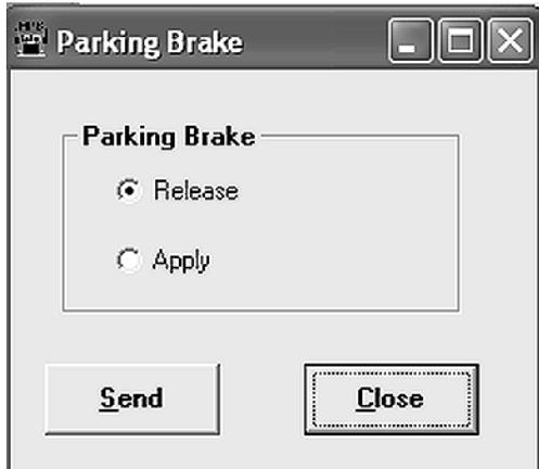
Select **Release** or **Apply**, then select **Send** to test the parking brake. Select **Close** to exit this screen.
