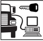
**NOTE:** TOOLBOX™ Software must be connected to the vehicle and the vehicle ignition must be ON in order to display information.
