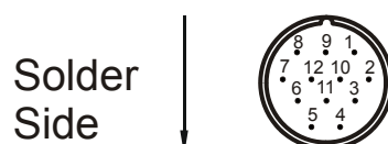
Fig. 31: View on RC series mating connector of the EnDat (internal thread M23)
