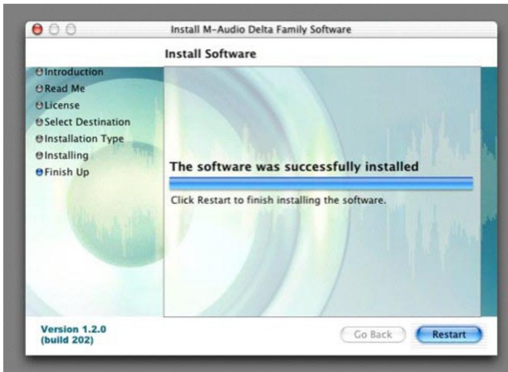
After the computer has rebooted, you may shut down the computer completely, disconnect your power cords, open the computer chassis and install the Audiophile 192 into an available PCI slot.
