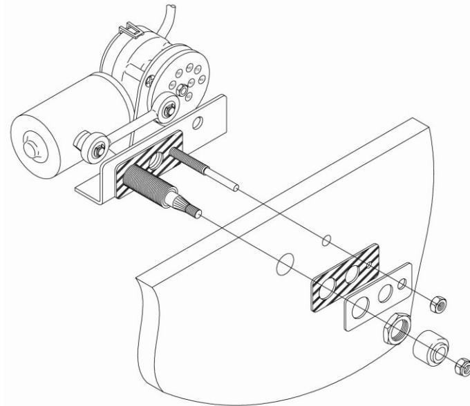
tightening torque :      25.6 Nm /      16.3 Nm /
