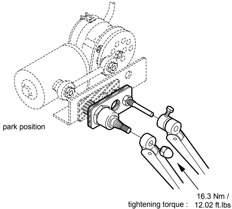
13. To complete the installation, the wiper must be enclosed by means of a panel or cover. Provide the wiper motor with sufficient ventilation.
