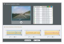
4 Move the control bar up/down to adjust the sensitivity range. If the range is wide, it is less sensitive, and if the range is narrow, it is more sensitive.
