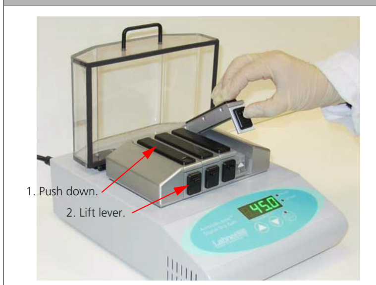
Figure 3.4 Opening the Clamps on the GeneAtlas™ Hybridization Station
