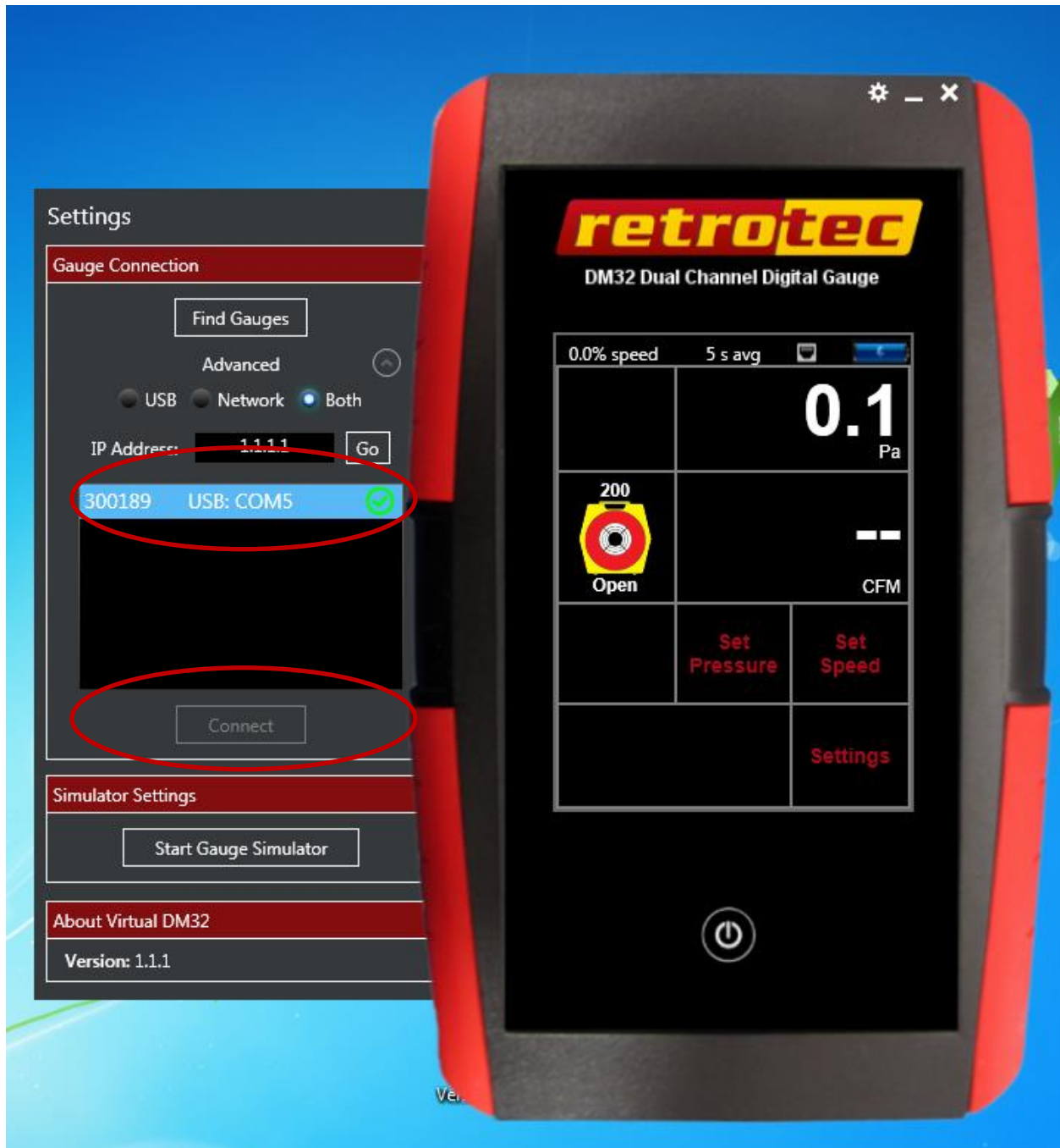
Figure 15: Select a gauge in the list and click [Connect] to start controlling a real gauge
