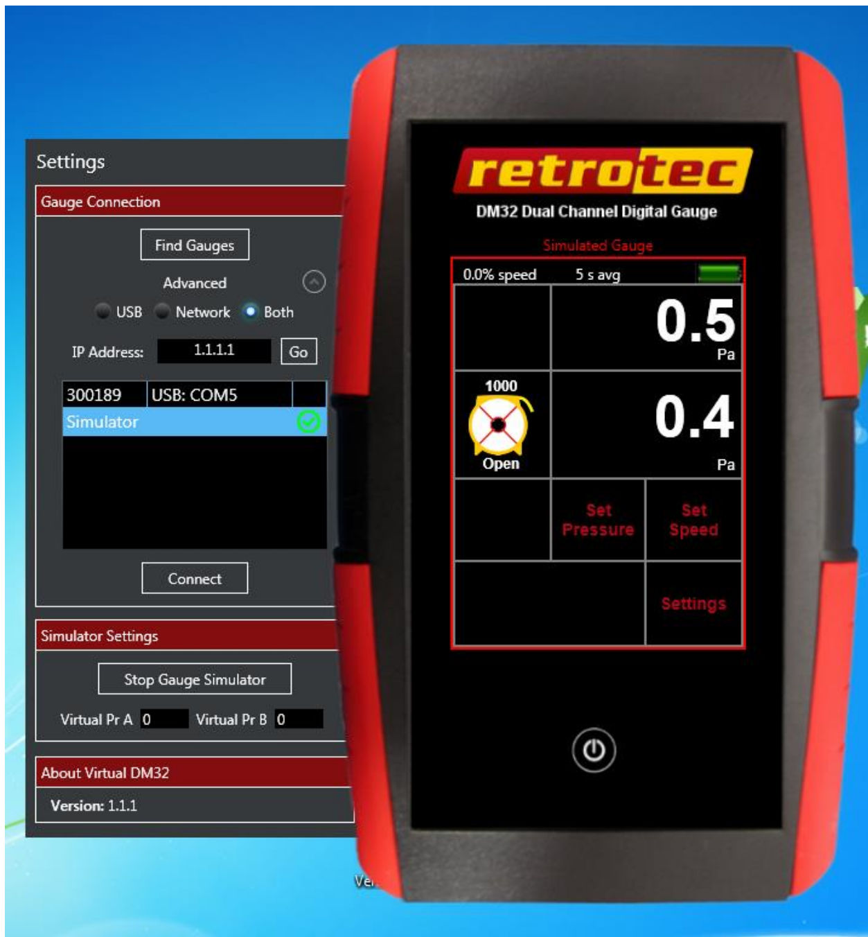
Figure 17: A simulated gauge is started and connected and is shown outlined in red on the virtual gauge screen
