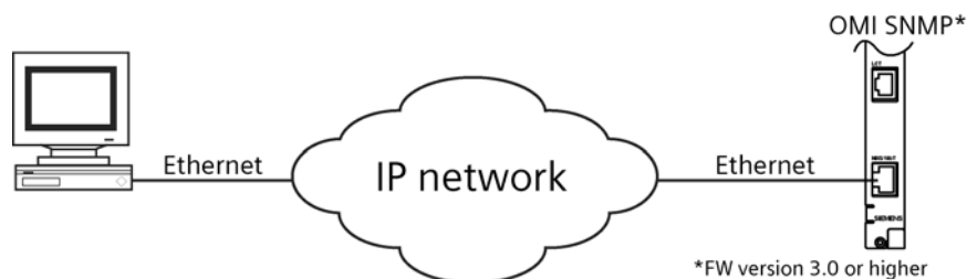
Fig. 2.296 LCT connected to an OMI SNMP
