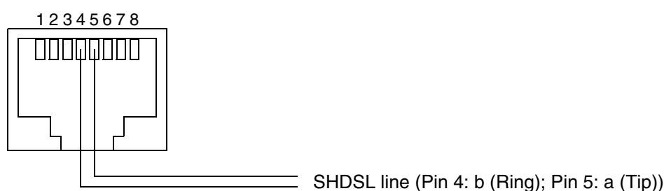
Fig. 2.59 RJ45 connector of the SHDSL interface
