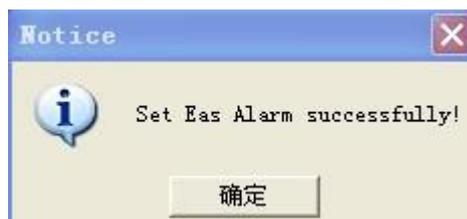
If failed, popup popbox, the failure reason may be the reader left the radio frequency or the access password is wrong.
